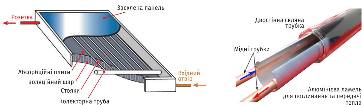
11. Figure - Structure of the flat plate and vacuum tube collectors (IS-SusCon project - http://howtobuildgreen.eu/ )
