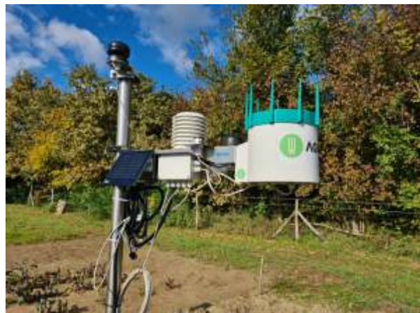
One of the installed meteorological measuring stations
