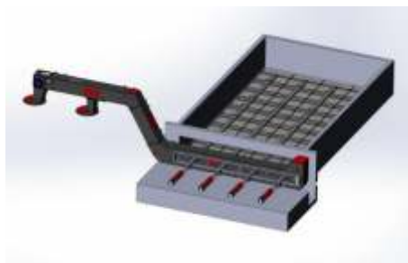
Image 2 – Composition of fuel “Live Bottom”
