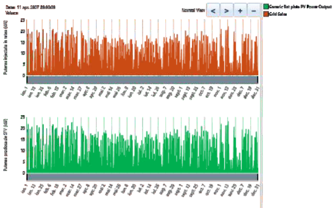
The electric power injected into the grid and the power produced by the photovoltaic system
